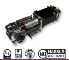
The MLRK1-JAC12 is a robust, straightforward field-installable motorized latch retraction kit for Jackson 1285/95, Kawneer 1686/1786, & AHT 8/9 series exit devices. It utilizes a CAT-designed custom assembly to maximize the pulling force. The only hole you'll need to drill is the raceway! It uses our new 1 TOUCH PTS "Push to Set" technology.
